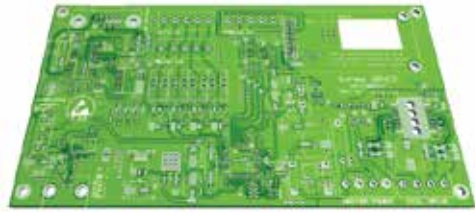
Figure 22. ARES PCB CAM Software 3D Visualization Output of PCB
