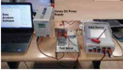
Figure 8. Complete Test Setup
