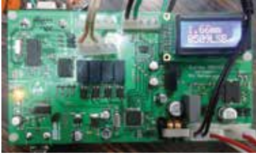
Figure 14. Realization of ECU on PCB
