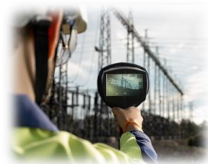
Figure 3. Acoustic Camera For Detecting PD
