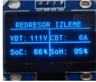
Figure 12. Measured Values Displayed on OLED
