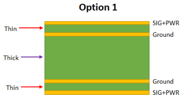
Figure 6. 4-Layer PCB Structure for Low EMI/EMC
