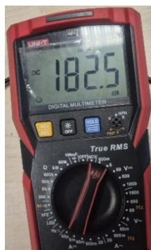
Figure 11. Amplified Voltage Output from Shunt Resistor
