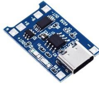
Figure 8. TP4056 Battery Charging System
