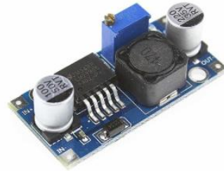
Figure 10. LM2596 Adjustable Step-Down Voltage Regulator Module
