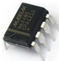
Figure 5. MAX485 Transceiver IC
