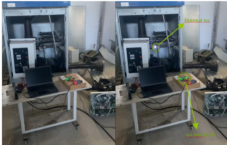
Figure 10. High Voltage Arc Tests in Laboratory Environment
