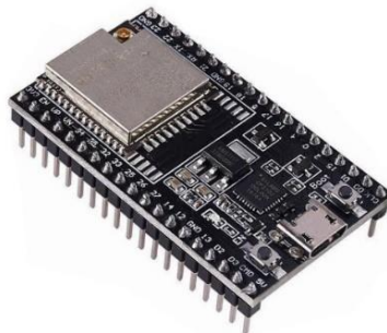
Figure 11. ESP32 Wi-Fi Communication Module
