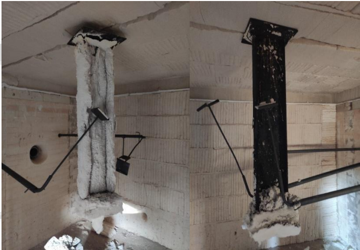
Figure 7: Specimens after the test, Product A is on the left and Product B is on the right
