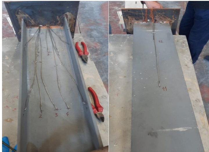
Figure 5: Fixed 12 thermocouples' locations for both Product A and B
