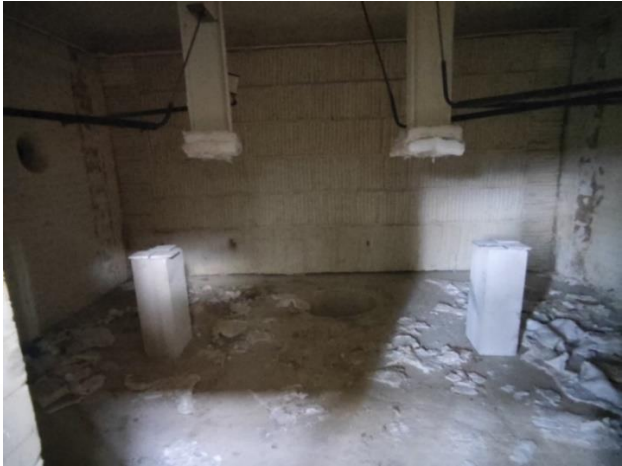
Figure 6: Specimens in the furnace just before the fire test
