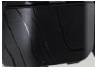
Figure 1. Car exterior trim calandra part made out of PC+ABS material
