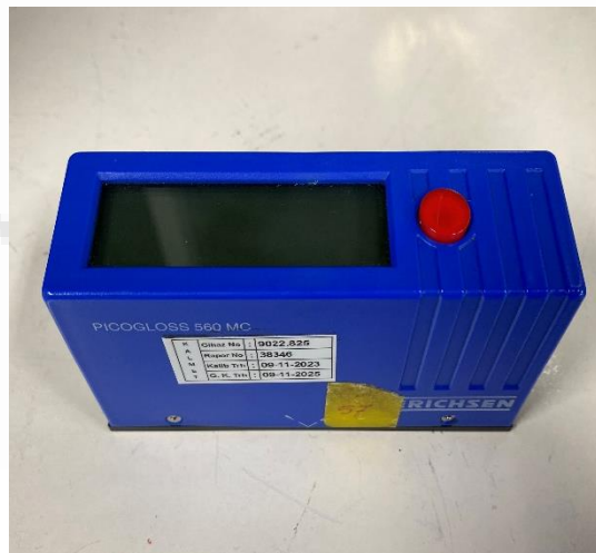
Figure 6. ERICHSEN PICOGLOSS 560 MC gloss measurment device that have been used for gloss measurement of the samples
