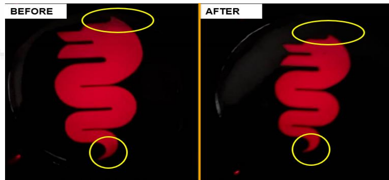
Figure 8. Air vent logo uniformity picture from mockup
