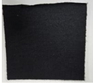
Figure 3. Car interior trim headliner part made out of polyester
