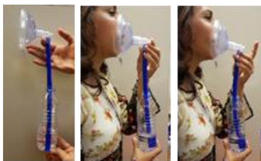
Figure 2: Trials with anesthesia masks combined with silicone tube
